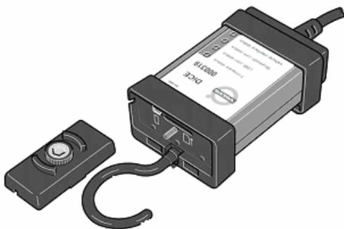
The inputs for USB and memory card<sup>1</sup> are located here.
